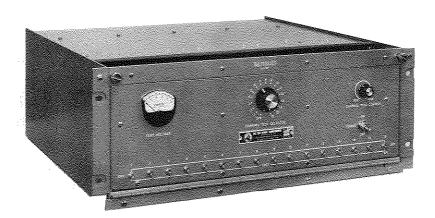
The Technical Material Corporation's Analog Data Control System is a solid-state device to electrically translate analog (infinitely-variable) voltages to digital information that may be readily transmitted over common communication circuits such as wire, cable or radio, including HF, VHF, UHF and Microwave links. On-off reporting and control is also available.
