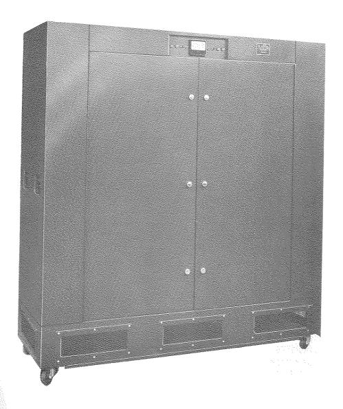
TMC Model TER-100K/50U, High Power Dummy Load, provides power dissipation of 100 kw average, 200 kw PEP, from 2-30 mcs with SWR not exceeding 1.5 to 1. Power and SWR ratio is indicated on a front panel meter.
