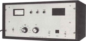
The TM-1000 Transceiver is a 1000-watt PEP device capable of operating between 1.6 and 26 MHz in up to eight pre-set channels. The standard model is designed to transmit in the CW, AME, USB and LSB modes and with selected options, can be automated through to the antenna. Although simplex operation is standard, eight-channel half-duplex is available on special order.
