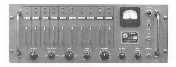
Technical Materiel Corporation Model VLR-1, Very Low Frequency Receiver, is a compact completely transistorized ten channel receiver providing exceptional stability, sensitivity, selectivity and reliability for the reception of continuous carrier, CW and FSK signals over the frequency range of 5 kc to 540 kcs. The tuning modules are designed to provide optimum reception under very weak signal conditions.
