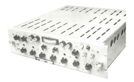
The Model LFE( ) Synthesizer/Exciter is the low frequency counterpart of the Model MMX for higher-frequencies. The LFE( ) covers all frequencies from 10 KHz to 1.9999 MHz in increments of 10 Hz. Like the MMX, it is simply necessary to set the desired mode of operation and frequency. Adjustable output in the mode desired is then instantly available. This all mode exciter function is self-contained in only 51/4" of panel space.
