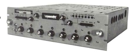
The TMC Model MMX-2 Series, Two Channel Independent Sideband Exciter is a compact all solid state unit designed particularly to accommodate the high capacity, multi-channel voice, teletype, data and FAX requirements of critical commercial and government point-to-point and tactical circuits. It is readily adaptable however to the less sophisticated single channel CW, USB or LSB requirements of back-up or other circuits where frequency allocations or operational needs dictate.
