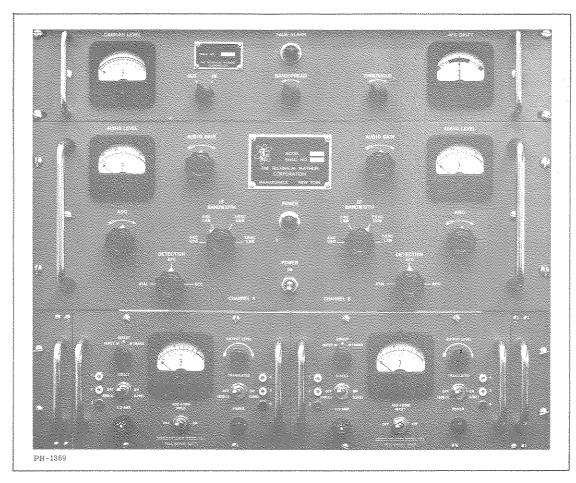
The TMC Models SBC sideband converters are IF type receiving adapters which will provide optimum reception of single, double, or independent SB signals, with or without Automatic Frequency Control. The AFC will function with up to 30 db carrier suppression and may be disabled for the reception of fully suppressed carrier signals.
