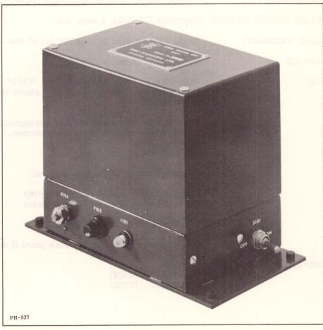
The TMC Model SCU is a Signal Control Unit designed to electronically control the stopping and starting of recording devices such as teleprinters, tape recorders and ink tape recorders.
