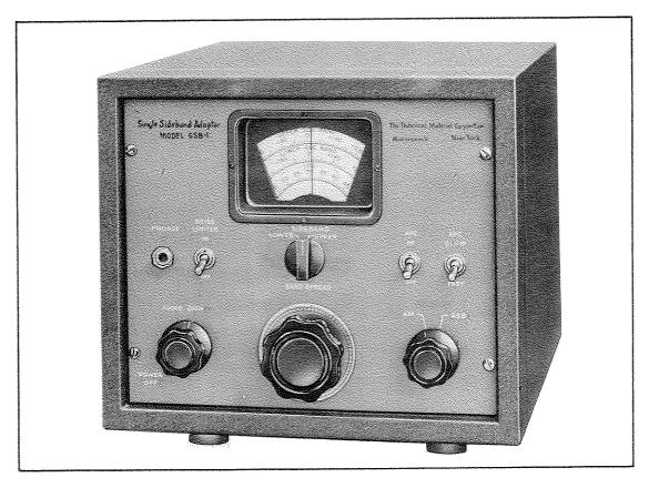
The TMC Model GSB, Single Sideband Adapter is a filter type slicer permitting accurate and simple tuning of SSB signals.
