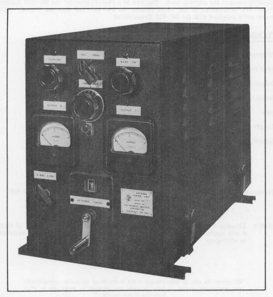
The TMC Antenna Tuning Unit, Model TAC-1, was specially designed for operation with the BC-610 Transmitter, but may also be used to match any transmitter whose output is 75 ohms to antenna loads of 50 to 1200 ohms over the frequency range of 2-18 Megacycles. The output loads may be either balanced or unbalanced.
