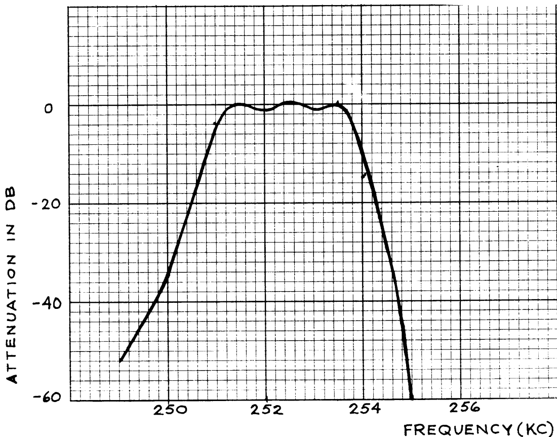
Figure 27. Frequency Response of FL1701
