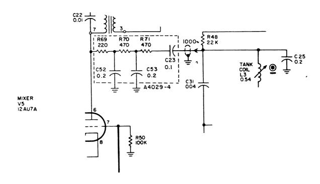
Simplified Schematic Correction Cut out and paste over appropriate area of figure 4-6, page 4-9 in TIS-3 manual.
