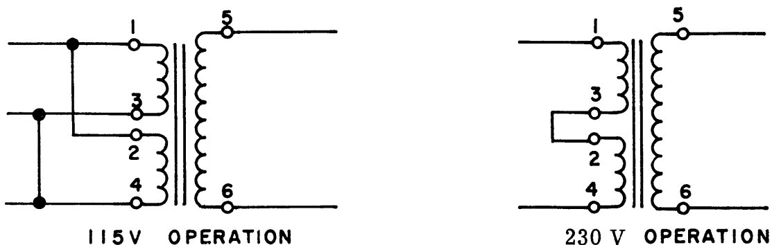
Figure 2-1. 115V to 230V Transformer Wiring Diagram
