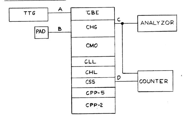
NOTE: Two-tone audio from TTG to channel 1 or channel 2 of the CBE. A single conductor shielded wire can be used for this purpose. TTG connections are as follows:
