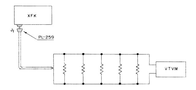
5 COMPOSITION RESISTORS: 360 △, 2W (RC42GF36IK) OR EQUIVALENT.
