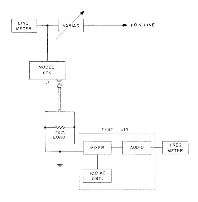
3.2.5.2. Frequency Stability Vs. Power Line Change Test.
