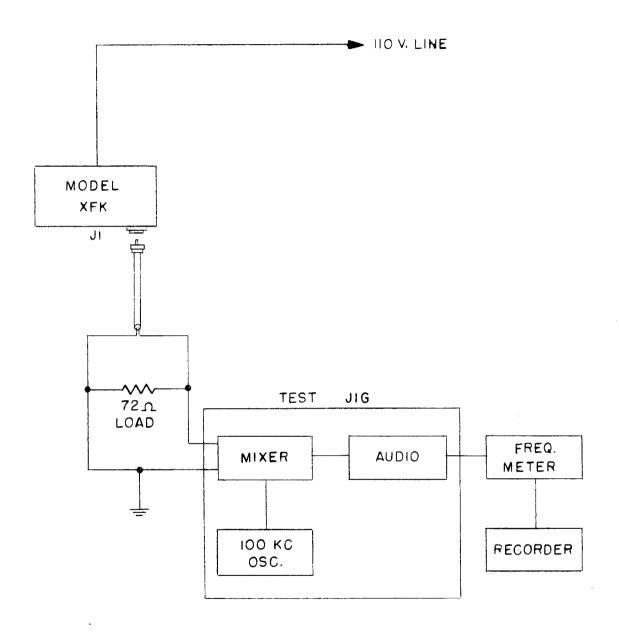
3.2.5.4. Frequency Stability Vs. Ambient Conditions Test.
