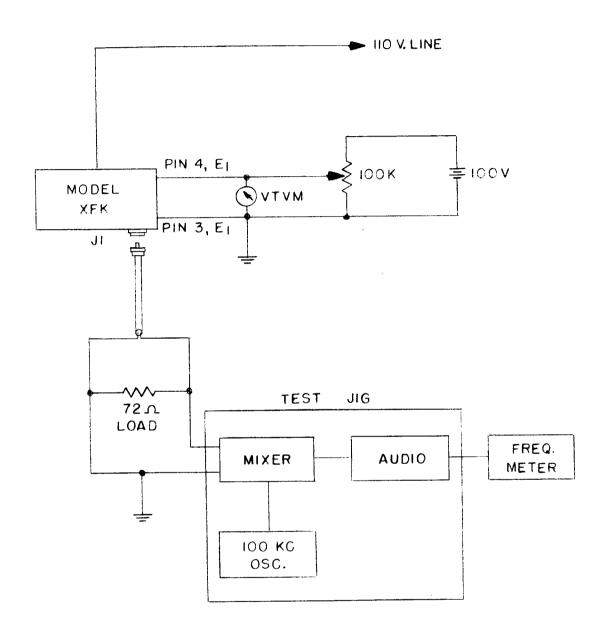
3.2.5.3. Frequency Stability Vs. Key Line Voltage Test.
