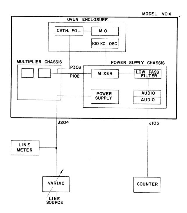
3.2.8.4 Master Oscillator Line Test Set-up.
