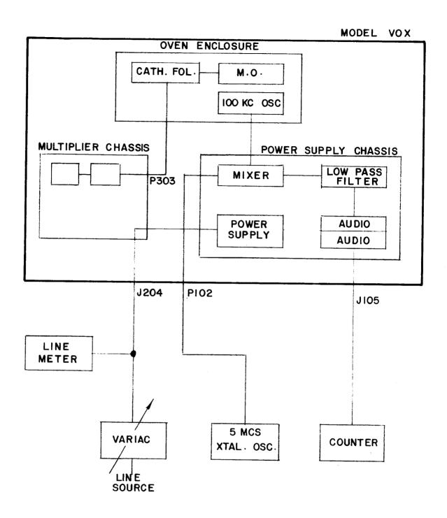
3.2.8.2. 100 Kcs. Oscillator Line Test Set-up.
