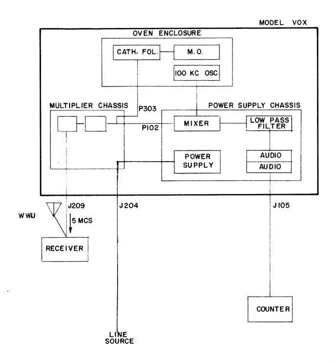
3.2.8.1. 100 Kcs. Oscillator Calibration Test Set-up.
