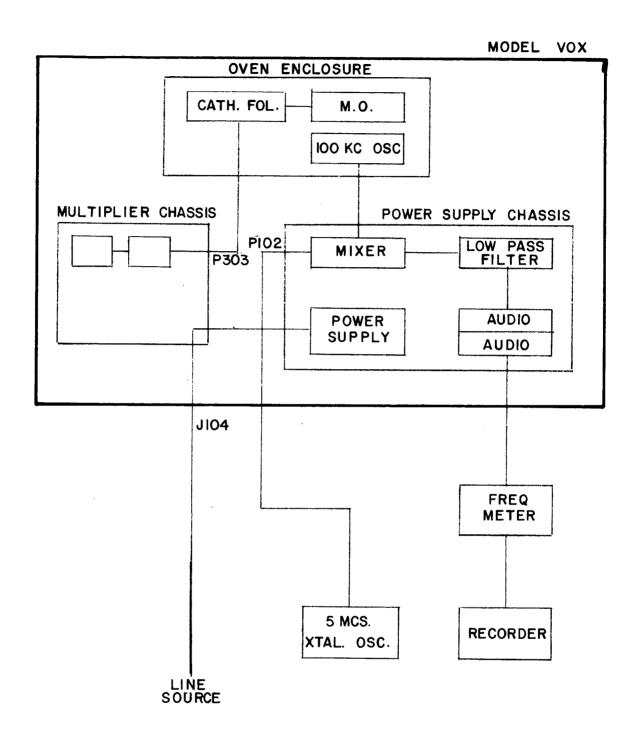
3.2.8.3. 100 Kcs. Oscillator Ambient Test Set-up.
