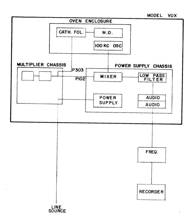
3.2.8.5. Master Oscillator Ambient Test Set-up.
