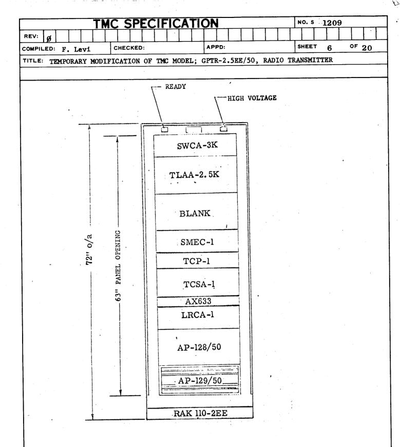
TMC MODEL; GPTR-2.5EE/50 RADIO TRANSMITTER
