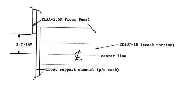
Fig. 6 Mounting of the "track" portion of TK 107-18.
