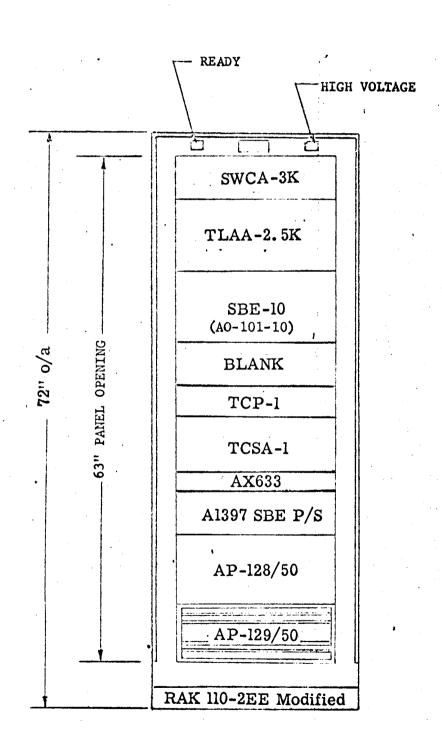
Fig. 9: TRANSMITTER AFTER MODIFICATION
