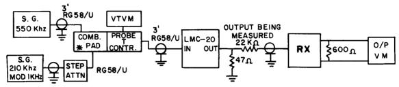
\* Combining Pad should match the output of the generator to the MC and should not attenuate 6db.
