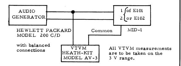
NOTE: Measurements taken at Terminal 1 of E101 to GROUND.
