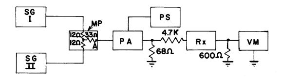
Inject two signals with a level of 250 mV each measured at the input jack J501 of the pre-amplifier: (point A)
