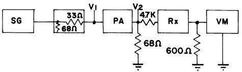
Inject a signal of 200 mV measured at the input J501 of the pre-amplifier. The signal should be 30% modulated at 1 kc/s.
