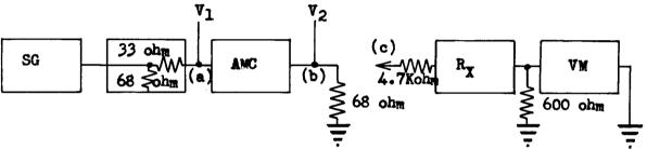
The 4.7 K ohm resistor is to prevent any serious change in the AMC termination when the detector is connected.
