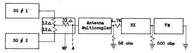
a) Inject two signals with a level of 250 mV each, measured at input jack J501: - (point A)
