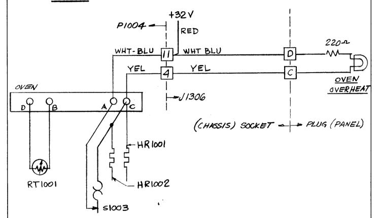
NOTE: This modification must be made in the HFR-LA and is, therefore, part of modification KIT-239. J1306, Pin 4, must be disconnected from ground and used for the YEL wire shown above. Pin 11, add WHT-ELU wire to the RED and follow through as shown.
