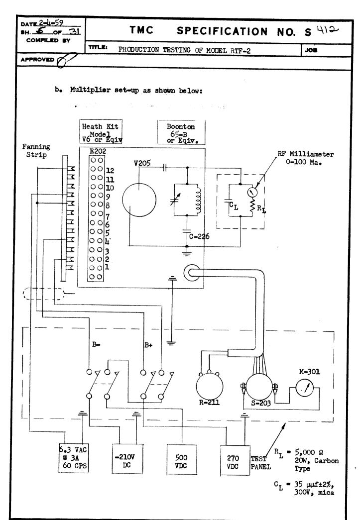
c. Alignment of Multiplier set-up as shown:
