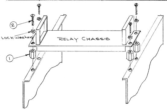
Step 1. Remove four screws holding Relay Deck and discard. (retain 4 lockwashers)
