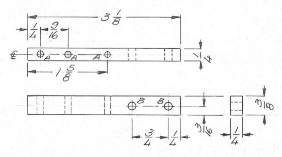
A HOLE - 1/8 DIA - 3 REQ. B HOLE - 5/32 DIA - 2 REQ.
