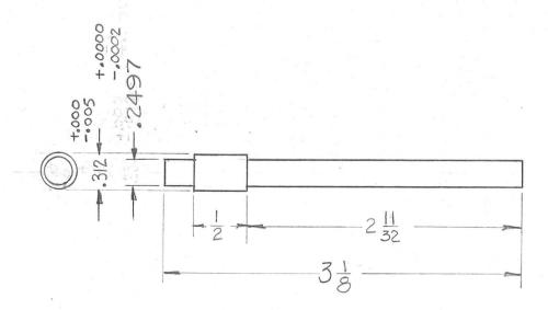
NOTE -ALL SHAFTS SHALL NOT DEVIATE FROM STRAIGHTNESS MORE THAN .005 PER FOOT.
