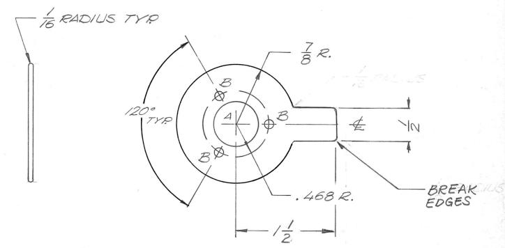
HOLE A 5/8 DIA. / REQ. HOLE B 1/8 DIA. 3 REQ.
