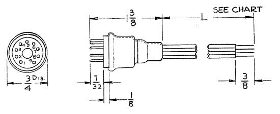
NC = No Connection All Leads will be Std. 22 Ga. Stranded Insulated Wire (Mil Type MWC22(7) U\_\_ Free End will be Stripped & Tinned 3"
