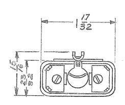
3 PRONG POLARIZED PLUG WITH REMOVABLE GROUND CONNECTION.
