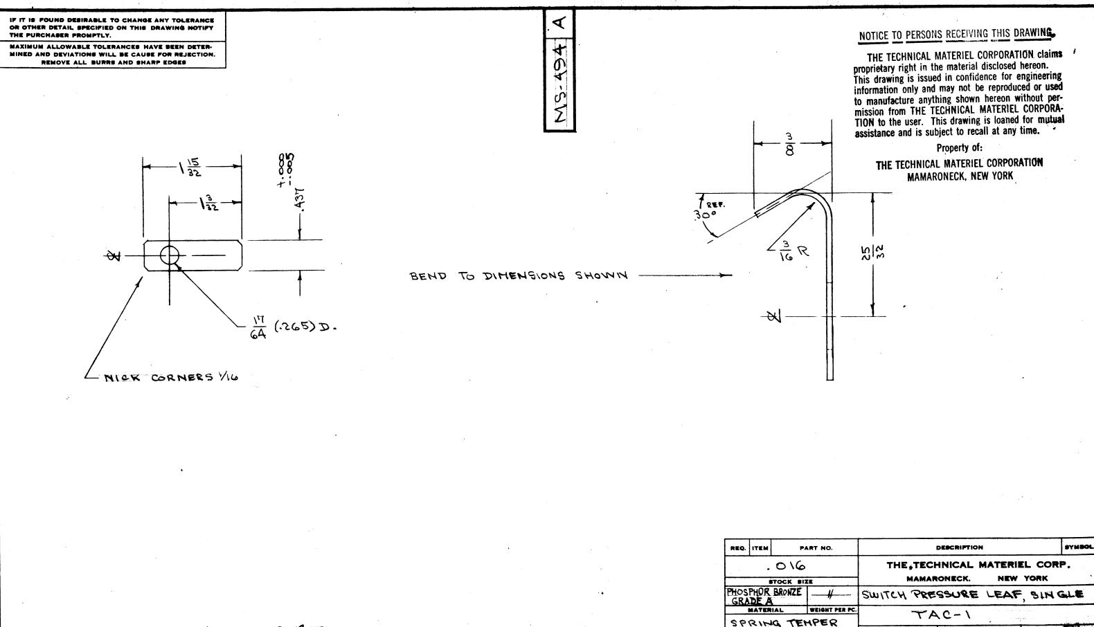
MAT'L WAS NICKEL SILVER 62061 5100 WAT. CN. NO. DRAFTS CHECKER ENG. APP DATE 12-29-53 135 A-666 TAC-1 DRILL, PUNCH, COMMERCIAL STOCK SIZES AND MANUFACTURERS MODEL PROJECT NO. ASS'Y. NO. DATE TOLERANCES ARE NOT INCLUDED. UED
