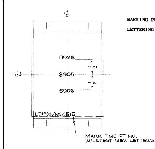
MARKING PROCESS: AS PER TMC SPECIFICATION S-727.
