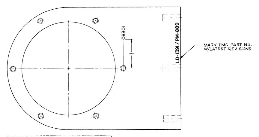
MARKING PROCESS: AS PER TMC SPECIFICATION 8-727.
