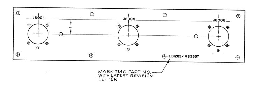
MARKING PROCESS: AS PER TMC SPECIFICATION S-727.
