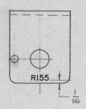
MARKING PROCESS: AS PER TMC SPEC S-727 LETTERING 1/8 HIGH BLACK GOTHIC, LOCATED AS SHOWN.
