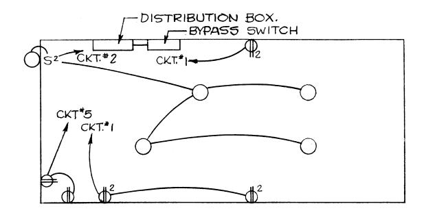
CKT. \* I - DUPLEX OUTLETS, 3 WIRE \* 12AWG - BLACK, WHITE & GREEN CKT. \* 2 - LIGHTING, TOP SWITCH INSIDE - BOTTOM SWITCH OUTSIDE CKT. \* 5 - 208V TWISTLOCK OUTLETS, 3 WIRE \* 10AWG - 2 BLACK, I GREEN BYPASS SWITCH TO DISTRIBUTION BOX, 3 WIRE \* 6.AWG - BLACK, GREEN & WHITE, CKT \* 1 & 2
