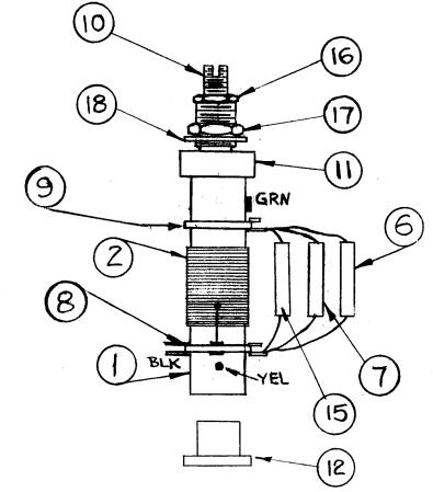
NOTE: KEEP CAPACITOR LEADS SHORT BUT DO NOT ALLOW ANY CAP TO TOUCH A LUG.
