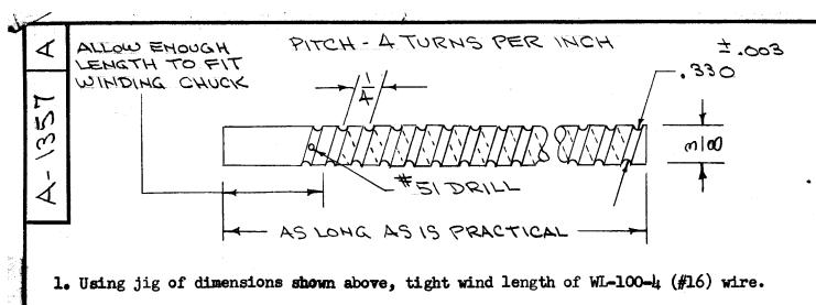
2. Screw jig out of wire leaving simple long coil of approximately .330 I.D.
