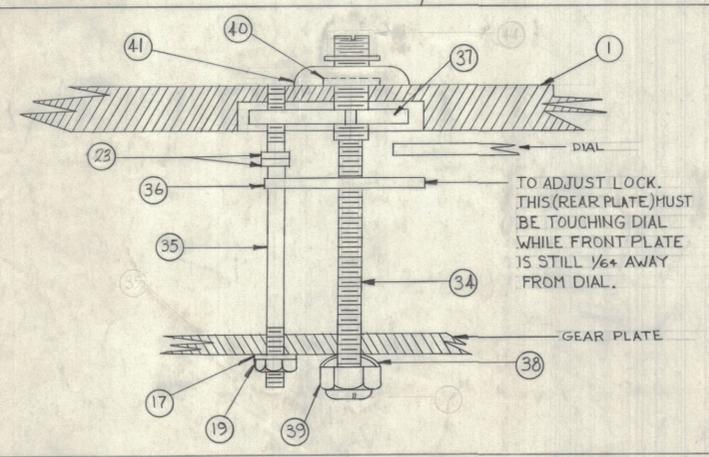
INSTALLATION & ADJUSTMENT DETAIL - DIAL LOCK ASS'Y.
