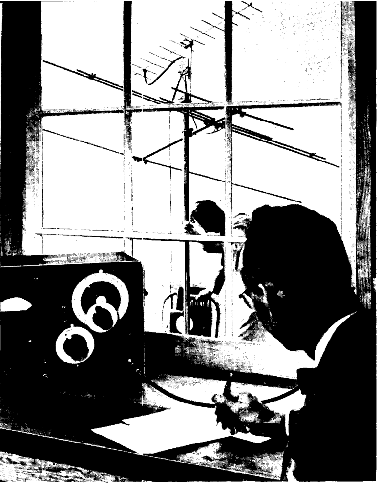
Checking television antenna performance on roof laboratory.
