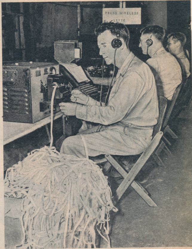
Technician operates transmitter which relays news flashes at 400 words a minute. Below, this control board on Long Island "talks back" to units overseas
