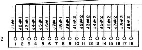
LOOP CIRCUITS D.C. OUTPUT TERMINALS (KEYED SIDE)
